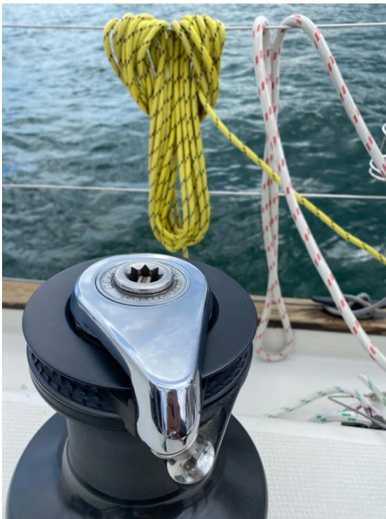
Photo of winch with 8mm and 15mm lines
