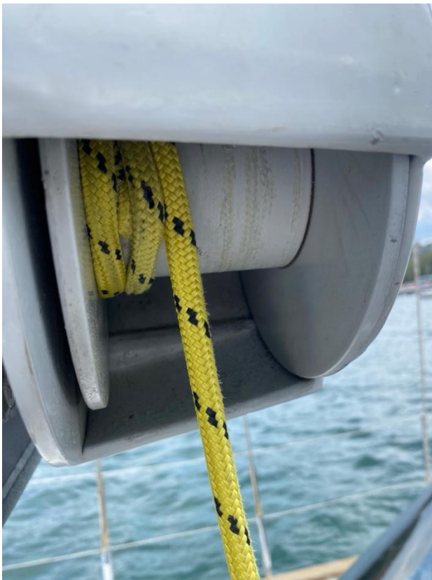
Photo showing the limited space inside the furling drum
